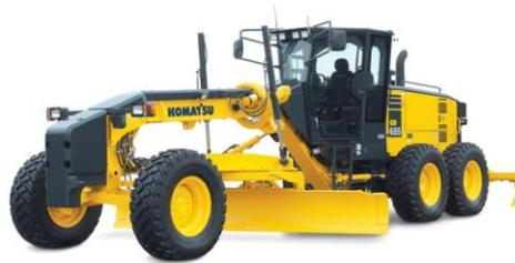
Gambar. 2.3 Motor grader
