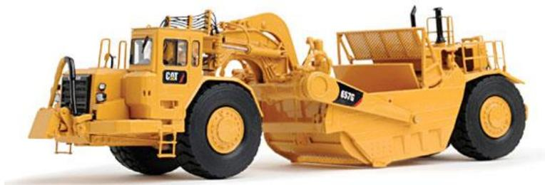
Gambar. 2.4 Wheel Tractor Scrapper
